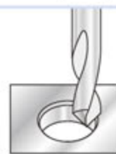
Hole chamfering machining
